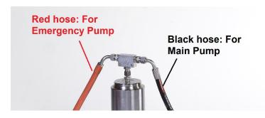
5. Manometers will be placed on 4 way hydraulic adaptor on Main/Emergency pumps
