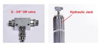
4. Black color flexible hose is to be attached to OR valve input (left side) and red color flexible hose is to be attached to OR valve input (right side)
